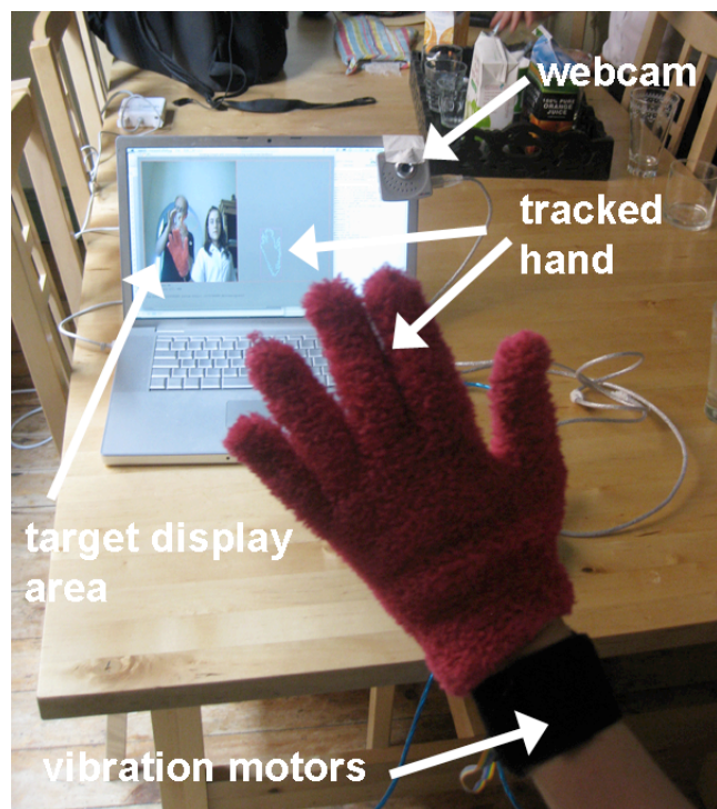
Figure 4. The experimental set up for testing whether two vibration motors could guide arm movements in one and two dimensions. The subjects wear a coloured glove on their moving hand that is tracked using a webcam and computer vision software. Subjects position their hand at a central starting point on the display area and then have to move their hand as quickly as possible to a target location. In some conditions the target position is shown with a brief visual cue. Vibrotactile feedback from two vibration motors provides information about the hand's proximity to the target in some of the test conditions.
