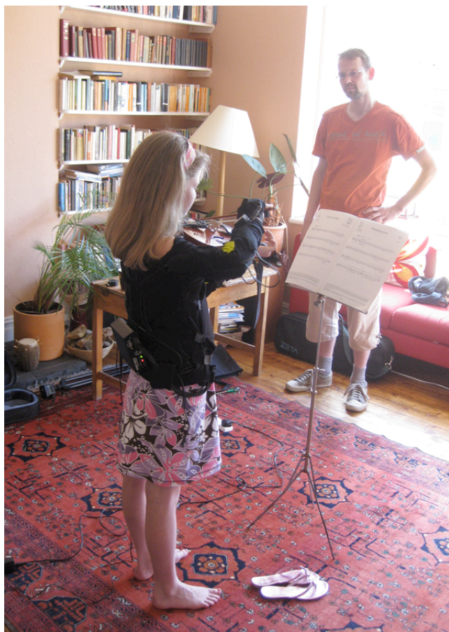
Figure 1. Tracking the bowing action of a young violin player who is wearing the Animazoo IGS-90-M motion tracking system. The movement of her bowing arm and the position of the violin are tracked using 6 inertial measurement units. The motion capture data are transmitted wirelessly to a
