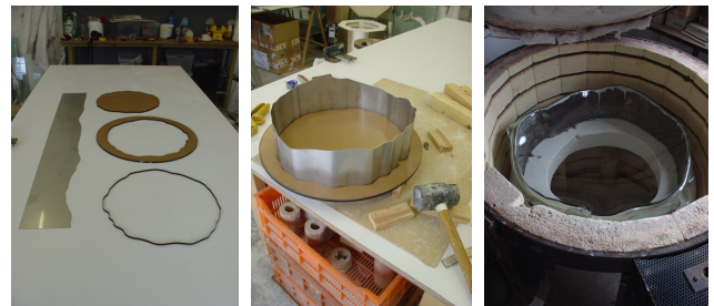
Fig. 5 The development of glass moulds from spatial data via laser cut profiles.
