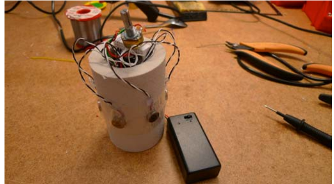
Figure 3: a grip with 7 vibrators, with manual control.
