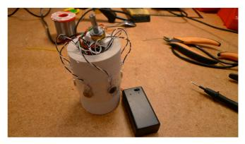
Figure 3: a grip with 7 vibrators, with manual control.
