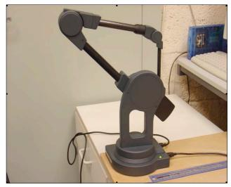
Fig 3. The G2 Microscribe digitising arm from Immersion Inc.
