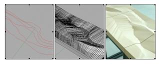
Fig. 2 Surface generation from recordings using the Shape-HandPlus data glove, illustrating the resulting aesthetic reflecting the movement of the designer's hand and fingers.
