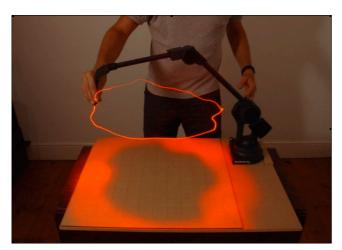
Fig. 4 Drawing/designing with the Microscribe G2
